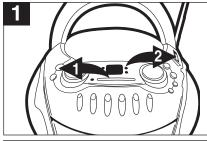
Press the POWER button **①** to the in position and slide the Function switch **②** to the CD position and insert a CD as described in the TO INSERT A CD section on page 6.
